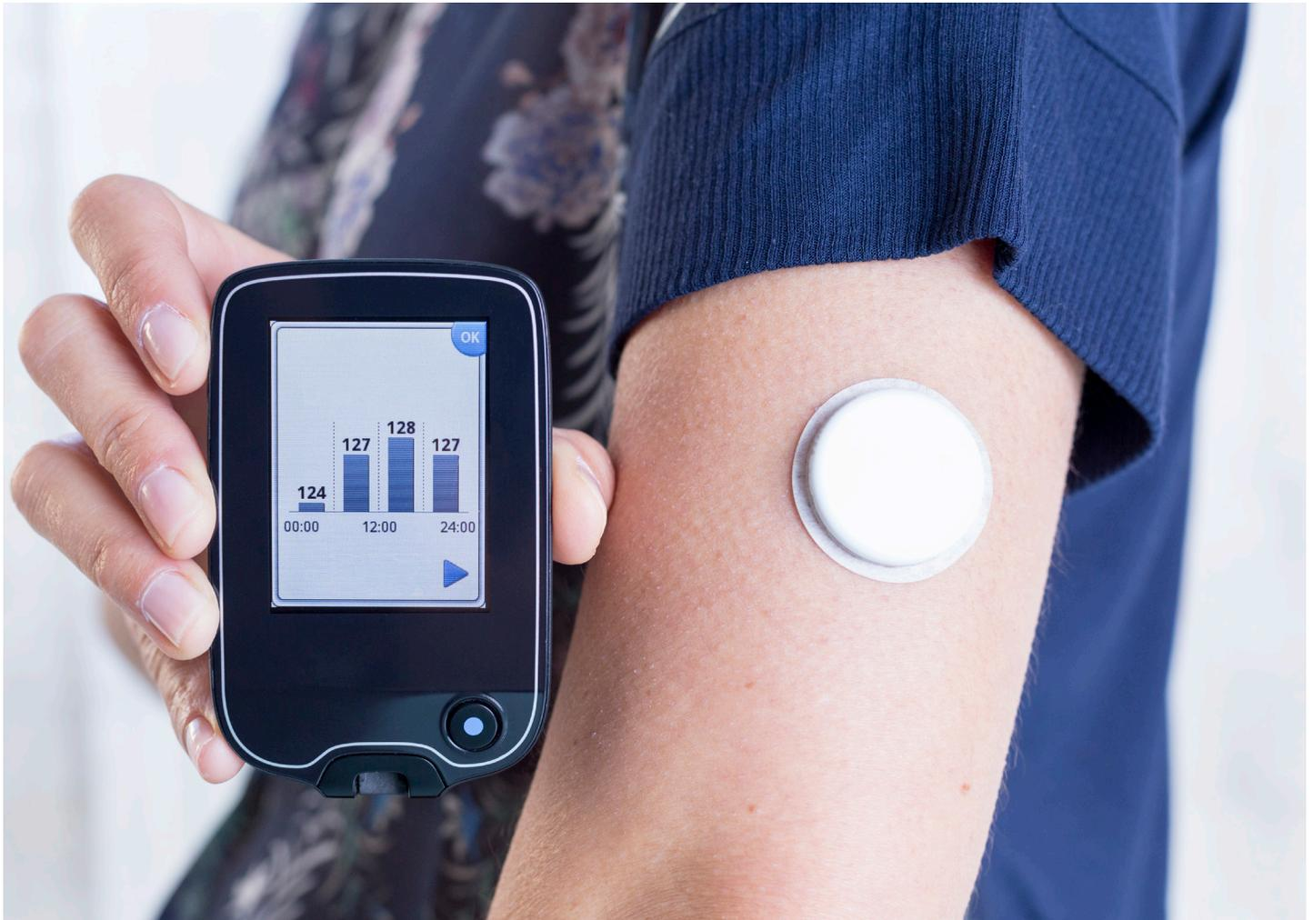
A flash glucose monitoring system uses an externally-worn glucose sensor with a small filament inserted under the skin of a person's upper arm. When the sensor is "flashed" or scanned with a separate
