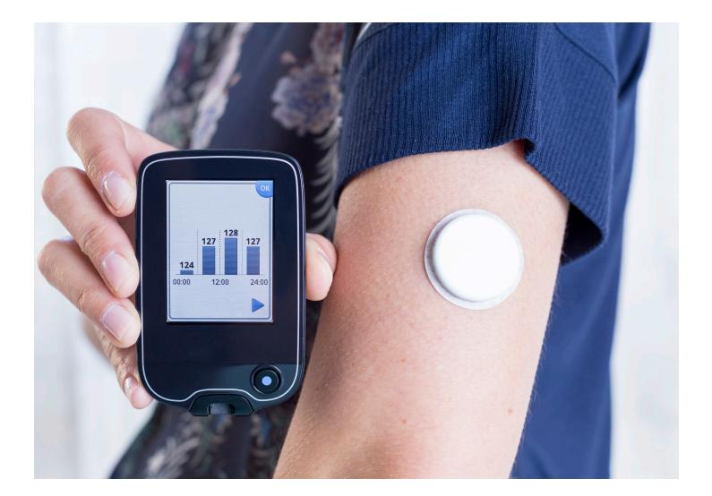
A flash glucose monitoring system uses an externallyworn glucose sensor with a small filament inserted under the skin of a person's upper arm. When the sensor is "flashed" or scanned with a separate touchscreen reader device, it transmits the realtime glucose reading and information on the most recent 8-hour trend to the reader. If the person with diabetes performs at least 3 sensor scans per day
